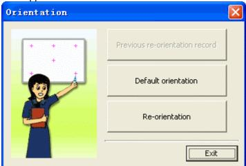
2) Left click "Re-orientation", it will open the Orientation window. Click center of the flashing sign" + " using electronic pen. Follow the prompt (there are six orientation points in all, left up, right up, right down, left down, top up and middle) as shown below:
